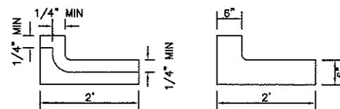
NOTE: CONSTRUCTION JOINT 10' SPACING SECTION VIEW OF CONSTRUCTION JOINT (SAW CUT ON SLABS HAND EDGE ON CURB & GUTTER)
